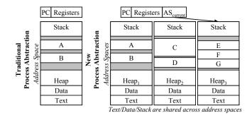
Figure 2: Contrasting SpaceJMP and Unix.
