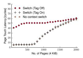
Figure 6: Impact of TLB tagging (M3) on a random-access workload. Tagging retains translations, and can lower costs of VAS switching.
