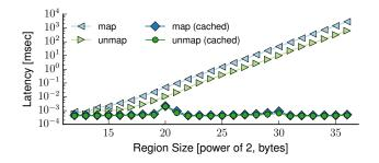
Figure 1: Page table construction (mmap) and removal (munmap) costs in Linux, using 4KiB pages. Does not include page zeroing costs.
