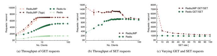
Figure 10: Performance comparison of Redis vs. a version of Redis using SpaceJMP
